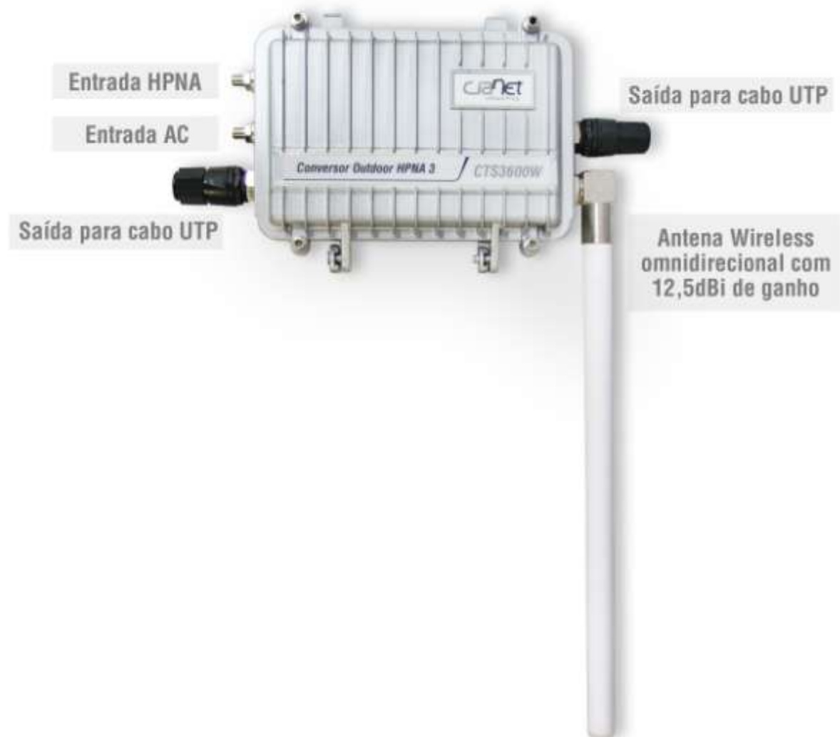
Figura 2.3-1: Conversor Outdoor HPNA 3 CTS3600W.
